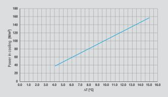
$\Delta T$  between reference ambient temperature and average water temperature = 10 K  $103~W/m^2$  (in accordance with EN14240)
